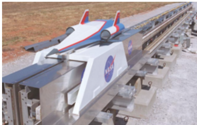
Different technologies to push a spacecraft down a long rail have been tested in several settings, including this Magnetic Levitation (MagLev) System evaluated at NASA's Marshall Space Flight Center. Engineers have a number of options to choose from as their designs progress: NASA
